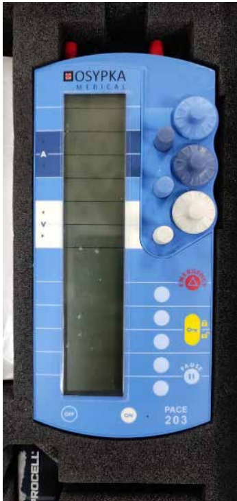
Dual Chamber Temporary Cardiac Pacemaker PACE 203 at B.Y.L. Nair Charitable Hospital, Mumbai
